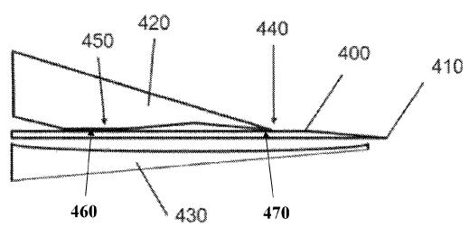
distance from said front edge than the clamping line. The clamp engages the knife blade along the clamping line and at the corresponding contact geometrical elements.
