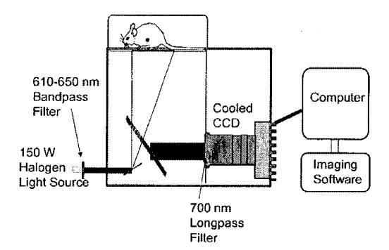
Figure 14. NIR Imaging Device
