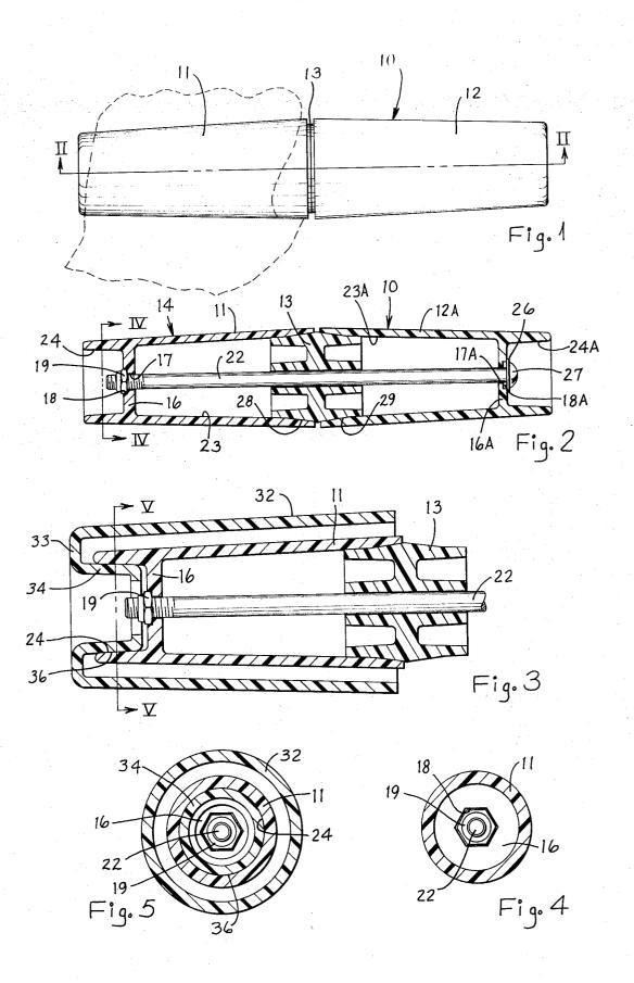
This invention relates in general to a device for use in exercising the hands, wrists and/or arms of a human being and, more particularly, to a type thereof in which the diameter of the manually gripped surfaces and the resistance to relative rotation thereof can be easily adjusted.
