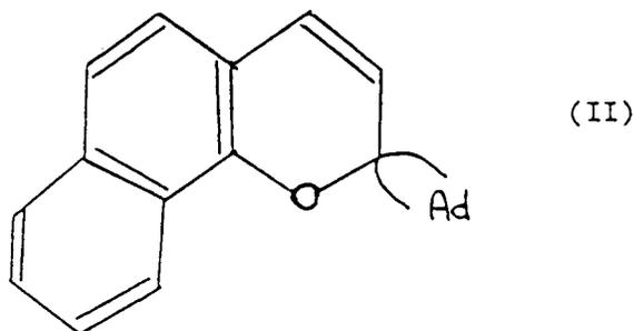
The final concentration of compound (II) was 1 kg per cubic metre. We have found that different photochromic compounds dissolve at different rates in the isocyanate, but the concentrations in the range 1-3 kg per cubic metre can be achieved without any problem. Optical data for a laminate incorporating compound (II) in polyurethane is given in Table I.
