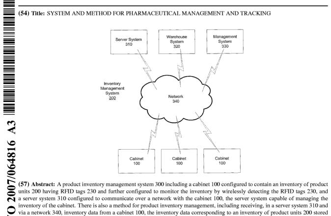
inventory of the cabinet. There is also a method for product inventory management, including receiving, in a server system 310 and via a network 340, inventory data from a cabinet 100, the inventory data corresponding to an inventory of product units 200 stored in the cabinet 100, and generating an order to have additional product units added to the cabinet according to the cabinet inventory.
