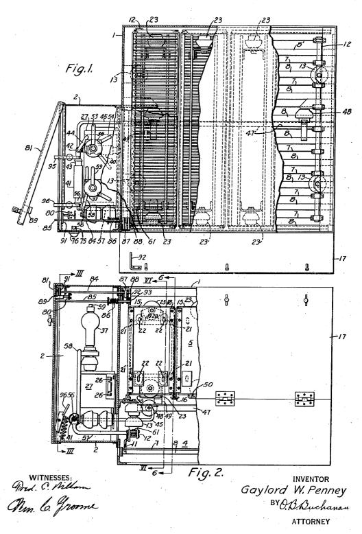
ELECTRICAL PRECIPITATOR FOR ATMOSPHERIC DUST
