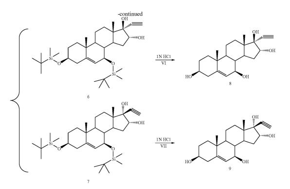
**[0254]** I: To a solution of 1 (1.0 g) and 0.56 g imidazole in 15 ml DMF, was added TBDMS-Cl 1.24 g, RT, o/n, work up with adding 50 ml water, solid show up, filtered out to yield white solid product 2, 1.75 g.
