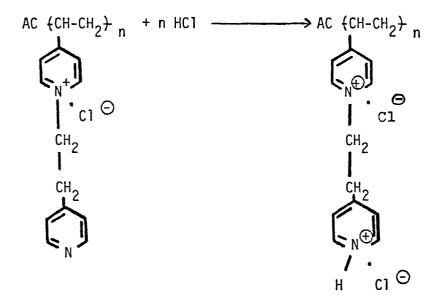
When a column was charged with the above-modified active carbon in the same manner as described in Example 5 and a model emulsified oil was passed through it to test the oil fraction removal ability of the modified carbon, it was found that the treated water discharged had a turbidity of 15 ppm and this value was maintained even after the passage of water for 250 hours. The crude water starting material had a turbidity of 80 to 120 ppm.
