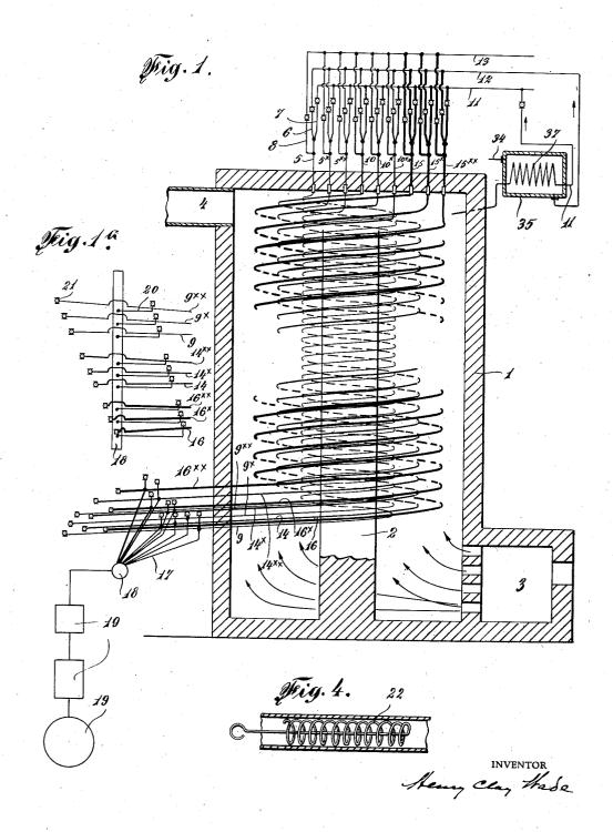
APPARATUS FOR HEAT TREATING HYDROCARBON OILS
