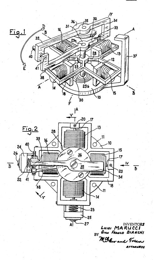
DIFFERENTIAL PNEUMATIC AMPLIFIER WITH ADJUSTABLE GAIN
