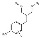
wherein  $R_1$  is a DMT group or a photolabile protecting group, a carbonate or a phosphate,  $R_2$  is H, a carbonate, phosphate or a thiol, A is H, a substituted alkoxy, alkyl, alkenyl, substituted aryl, amine or carboxylic acid and
