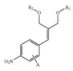
**[0082]** wherein R1 is a DMT group, a photolabile protective group, a carbonate or a phosphate, R2 is H, a carbonate, phosphate or a thiol, A is H, a substituted alkoxy, alkyl, alkenyl, substituted aryl, amine or carboxylic acid and
