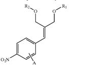
**[0121]** In formula II,  $R_1$  is a DMT group, a photolabilte protecting group, a carbonate or a phosphate,  $R_2$  is H, a carbonate, phosphate or a thiol, A is H, a substituted alkoxy, alkyl, alkenyl, substituted aryl, amine or carboxylic acid.
