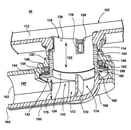
that is less than or equal to the cross-sectional area of the bearing inlet. The deflector is also aligned with the bearing inlet and defines a turn in the supply outlet for directing liquid into the bearing inlet.
