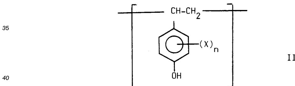
where X denotes a halogen atom and n denotes zero or 1, and copolymers having units of formula II together with units derived from at least one other vinyl monomer, preferably styrene or an alkyl or hydroxyalkyl acrylate or methacrylate such as methyl methacrylate or 2-hydroxyethyl methacrylate, the polymers having a weight average molecular weight of 1500 to 50,000, particularly 2000 to 30,000.
