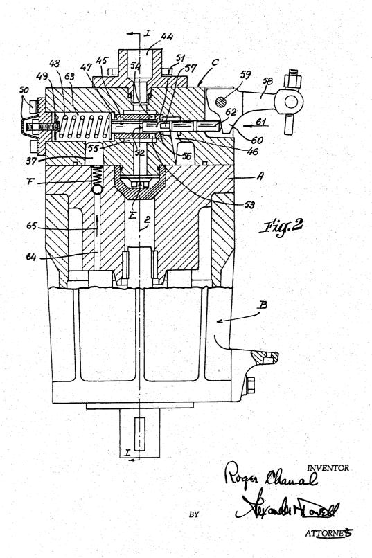
SWASH PLATE HYDRAULIC PUMPS HAVING AXIALLY DISPOSED PISTONS
