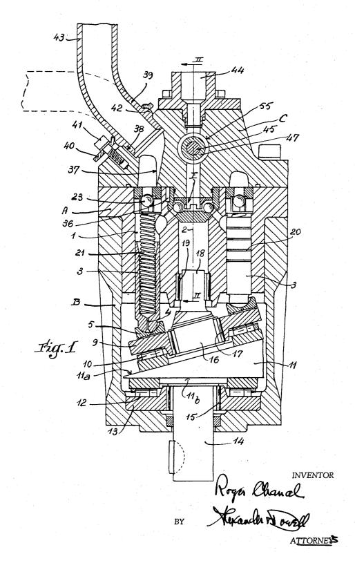
SWASH PLATE HYDRAULIC PUMPS HAVING AXIALLY DISPOSED PISTONS
