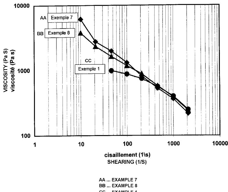
(57) Abstract: The invention concerns copolyamides obtained by using multifunctional monomers. It consists in using at least one multifunctional monomer comprising at least three reactive functions and at least another multifunctional monomer, in amounts such that the terminal group concentrations are balanced. The copolyamides are more particularly high viscosity copolyamides. The invention also concerns compositions based on said copolyamides.
