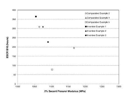
(57) Abstract: A dual reactor solution process gives high density polyethylene compositions containing a first ethylene copolymer and a second ethylene copolymer and which have good processability and ESCR properties. The polyethylene compositions are suitable for compression molding or injection molding applications and are particularly useful in the manufacture of caps and closures for bottles or containers.
