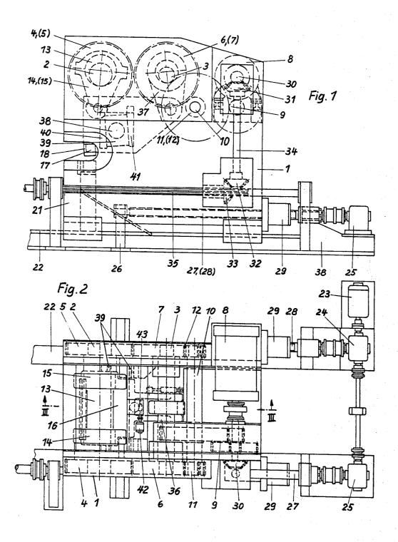
SHEARS FOR TRIMMING THICK METAL SHEETS OR PLATES
