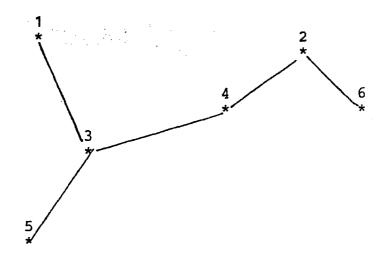
The exemplified configuration can be given various branch systems depending on desired synchronization routes. The task of the paging network unit is simply to define a branch system that is branched as much as possible and the number of successive branches is minimized. As indicated in our example, the configuration of fig. a) is preferable to that of fig. b) since synchronization can be performed with only 2 sequences: 1.: 3-4, 3-1, 3-5, 2.: 4-2, 4-6.
