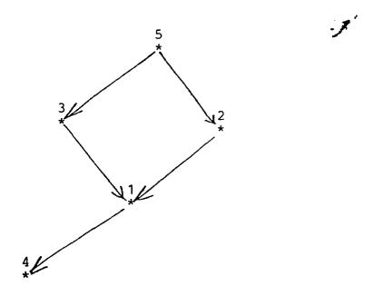
It is necessary to presume in our example that the rest of the network configuration is such that the route of synchronization proceeds just via station No. 5.
