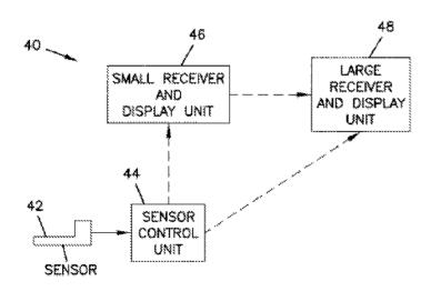
(57) Abstract: Devices and methods for positioning a portion of a sensor at a first predetermined location, displacing the portion of the sensor from the first predetermined location to a second predetermined location, and detecting one or signals associated with an analyte level of a patient at the second predetermined location are disclosed. Also provided are systems and kits for use in analyte monitoring.
