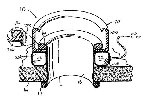
(57) Abstract: An adjustable surgical wound retractor (10) having outer and inner resilient rings (14, 16) connected together by a flexible sleeve (18). The outer ring (14) may be rolled down onto the sleeve (18) for coarse adjustment of the sleeve (18) length suitable for initial installation in an incision. A lifter (20) interposed between the outer surface around the incision and the outer ring (14) provides a fine adjustment. The lifter (20) may be actuated pneumatically or mechanically.
