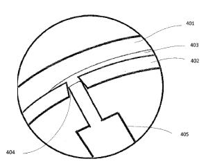
(57) Abstract: The present invention relates generally to methods of fabricating an electro-active optical structure, such as an electro-active lens or an electro-active lens blank. In some embodiments, the invention relates to fabrication methods that comprise an improved process for delivering an electro-active material into a cavity, resulting in electro-active structures that can be manufactured in less time and with lowered costs.
