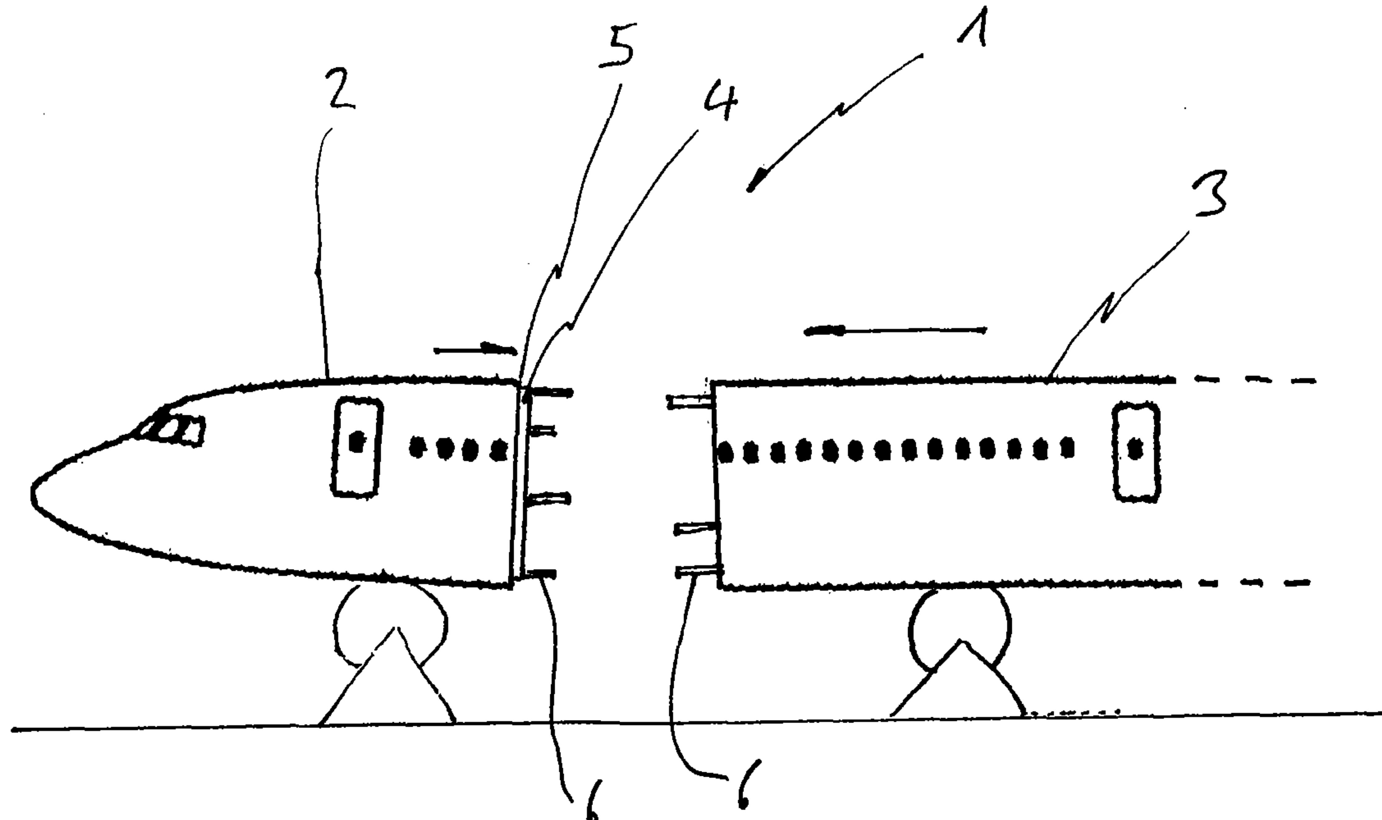
(57) **Abstract:** The present invention relates to a method of preparing the connection of two fuselage sections (2, 3). A less complicated and time consuming method was found by using High-Speed-Drilling (HSD) for a group of final bore holes through the outer skin of at least one fuselage section and/or the coupling means using one drilling template preferably without any pilot drilling.
