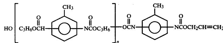
where n is an integer wherein the molecular weight is equal to 1000, in a thickness in the range of 0.5 mils to 2.5 mils and cured with ultraviolet light for 60 seconds. The coated sheets are tested as described in Examples 1 30 and 2. The results are set forth in Table I.
