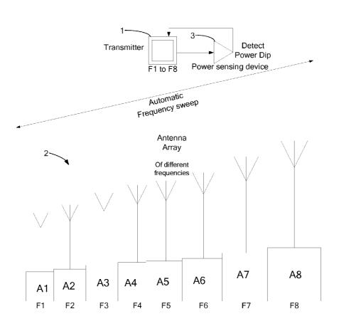
When the transmitted frequency equals the resonant frequency of any antenna, a power dip in the transmitted power will be detected
