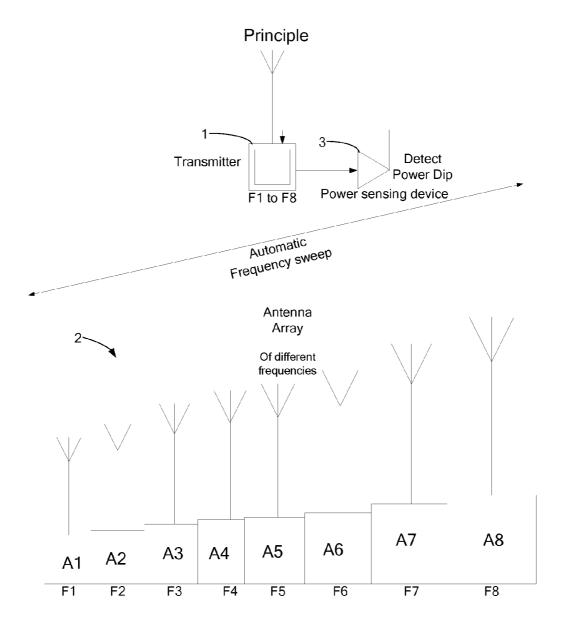
When the transmitted frequency equals the resonant frequency of any antenna, a power dip in the transmitted power will be detected
