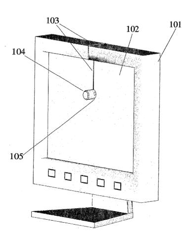
(57) Abstract: An apparatus for reducing gazeperception discrepancies while video teleconferencing, consisting of a camera mounted directly on a display screen, and preferentially along the same axis as the line of sight between the local user and the remote user's eyes as displayed on the display screen.
