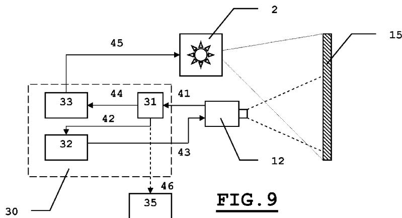
(57) Abstract : The invention relates to a method for controlling the power of a light source of a device comprising an interactive facade, on the basis of images captured by the facade. The invention also relates to designing and adapting a device such as an interactive display case or vending machine using said method.
