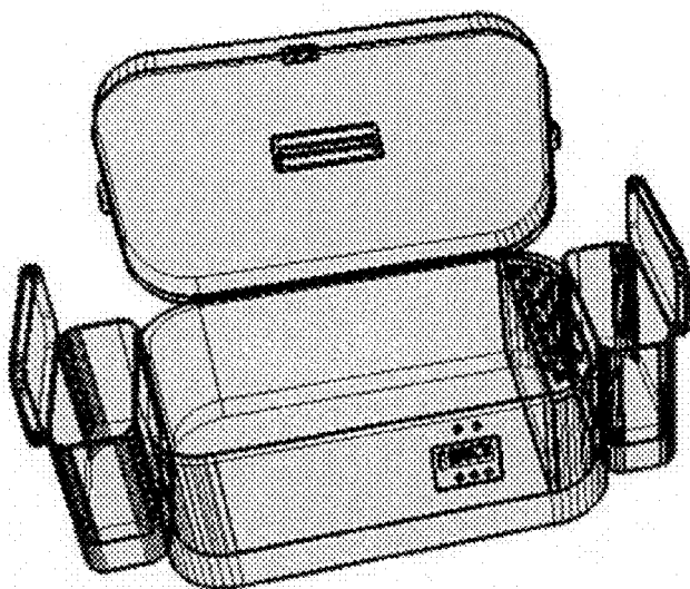
Figure 8: A diagram for the Mini-incubator with a special design (2 additional compartments as a safe storage for the Carbogen gas cylinder and other accessories).
