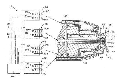
(57) Abstract: A spray applicator cleaning system and a method includes a valve and control means (12) for discharging air and solvent in alternating bursts to shaping air nozzles (60, 62, 94), a coating supply (34) conduit and a dedicated cleaning nozzle (94) on the applicator (10).
