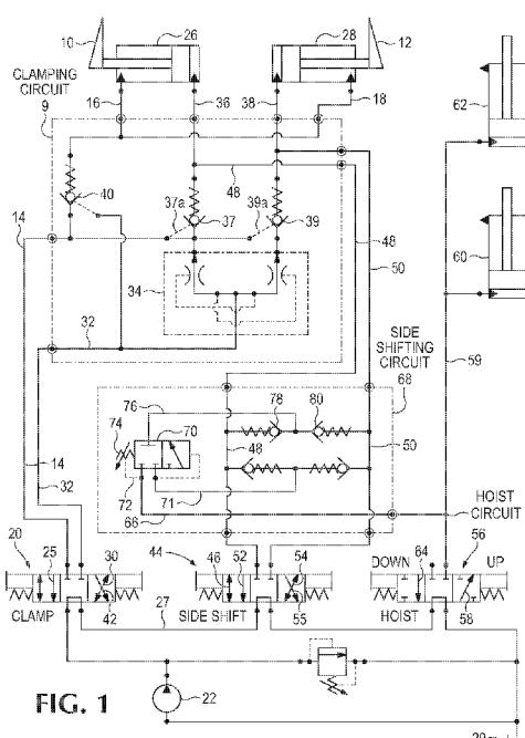
**(57) Abstract:** Different exemplary control systems for a hydraulically powered load-handling clamp, of the type usually mountable on industrial lift trucks or automatically guided vehicles, are disclosed. The disclosed systems variably limit a hydraulic force, by which load-clamping arms move a load substantially transversely, automatically depending on the weight of the load being moved, so as to avoid excessive transverse force applied to fragile loads.
