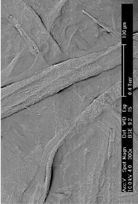
d. BSE image of a sheet coated with 3.1 g/m² MFC+A starch
