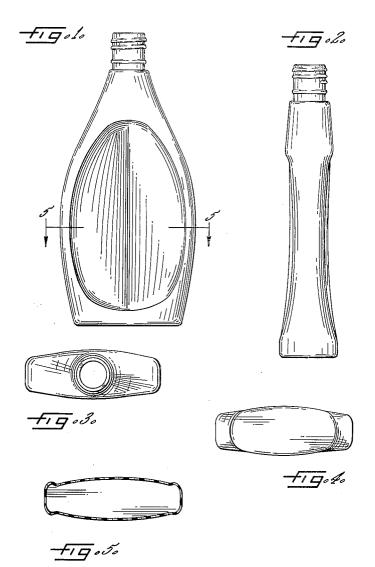
FIG. 1 is a front elevational view of a bottle illustrating my new design;
