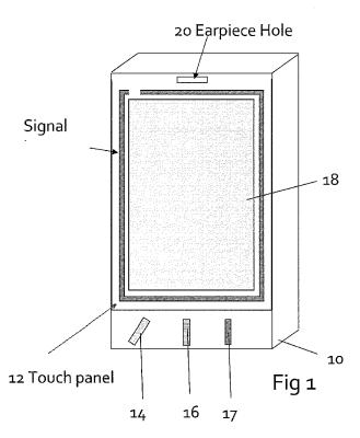
(57) Abstract: An apparatus comprising a display component comprising at least one display part and an electrically conductive part electrically isolated from the at least one display part.
