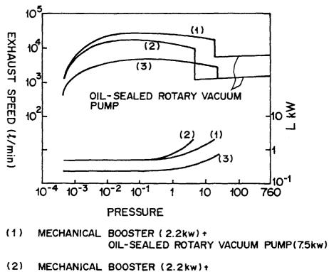
OIL-SEALED ROTARY VACUUM PUMP (2.2kw)
