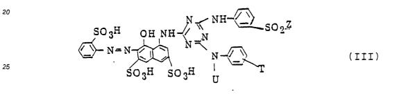
wherein U is a hydrogen atom, a methyl group or an ethyl group, T is a hydrogen atom, a chlorine atom or <sup>30</sup> a bromine atom, and Z is as defined above.
