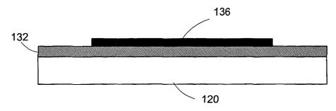
(57) Abstract: A sacrificial layer and a method for applying said sacrificial layer in fabricating microelectromechanical devices are disclosed herein. The sacrificial layer comprises an early transition metal. Specifically, the sacrificial layer comprises an early transition metal element, an early transition metal alloy or an early transition metal silicide.
