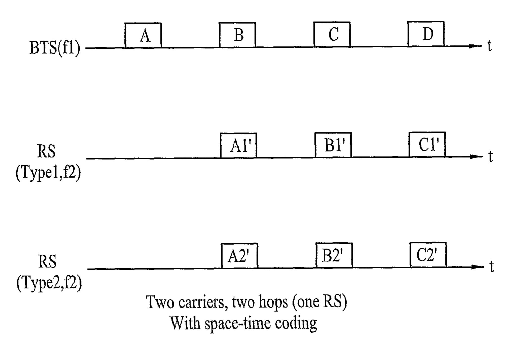
(57) Abstract: A method of identifying a space-time encoded signal in a wireless communication system having at least two different decoder types is disclosed. The method includes receiving at least one pilot signal from a transmitting end, wherein the pilot signal is represented by either Type 0 or Type 1, determining which of Type 0 or Type 1 is represented in the received pilot signal, and activating the space-time decoder for performing space-time decoding, if the pilot signal is Type 1.
