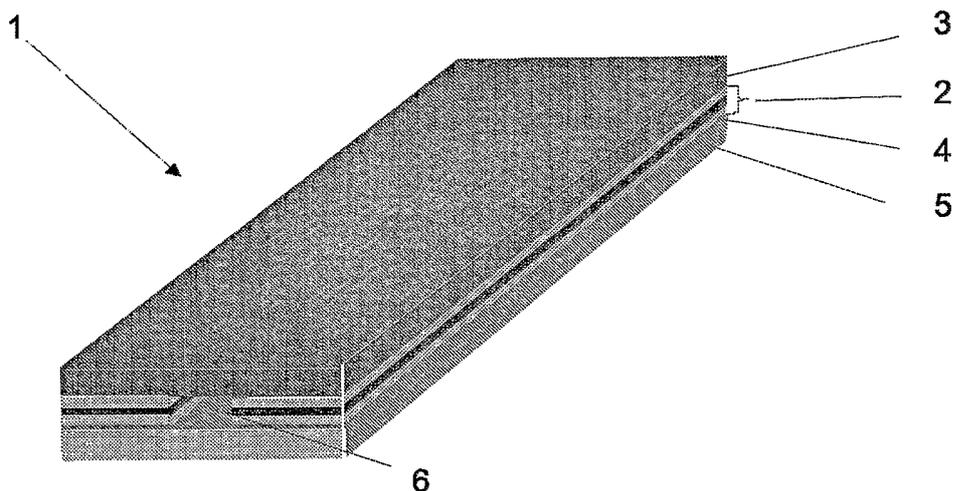
(57) Abstract: The invention relates to the use of a film for medical diagnostic strips by means of which biological liquids are tested. Said film comprises a carrier material the one or two faces of which are hydrophilized by chemical treatment and said treated surface has the following properties: permanent hydrophilic properties; a surface tension of at least 58 mN/m and a contact angle with water smaller 50°.
