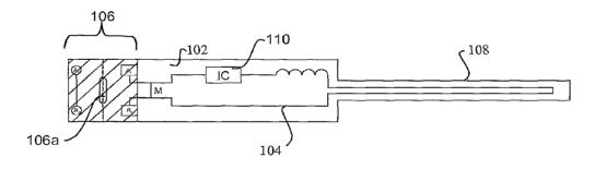
(57) Abstract: A tamper evident RFID circuit uses a fold section that forms a capacitive element when folded together.
