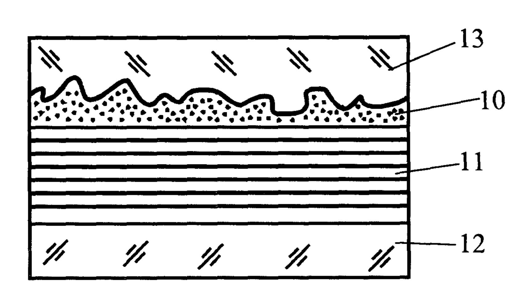
(57) Abstract: The present invention relates to a new optical component comprising an anisotropic diffuser (5,10) with patterned anisotropy; and means (9, 11, 14, 16, 17, 20, 21, 30, 32) for providing a colourshift observable upon changing viewing angle (6) and/or changing angle of incident light (2). It also relates to methods for making such an optical component and uses of such optical components as security elements with a very high level of security.
