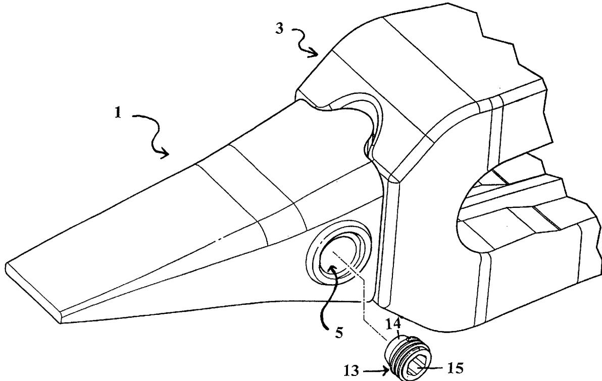
**FIGURE 1** WEAR MEMBER WITH PIN-RETAINER RECEIVING HOLE
