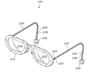
(57) Abstract: The eyeglasses (105) have a lens frame (215) in which lenses (210) are mounted. Proximal ends of flexible temple members (230) are removably attachable to opposite sides of the lens frame (215). The temple members (230) are sized to extend over and behind the ears to the vicinity of the ear lobe. A counterweight (240) is attached to the end of the temple members (230) by a releasable fastener. The releasable fastener may be a clasp (225) and a complementary receiving member.
