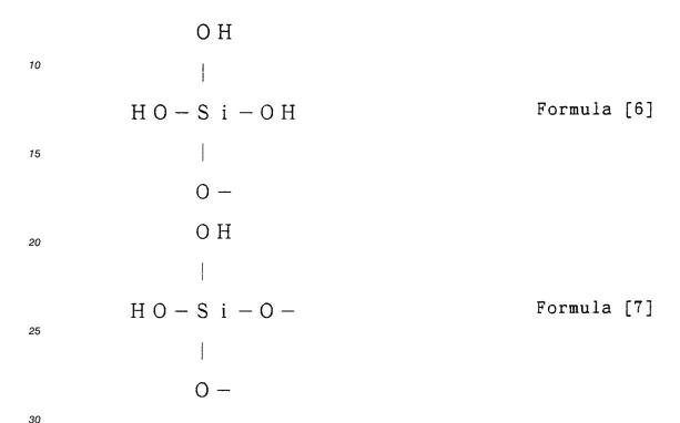
The monomolecular film (inner layer) obtained in this way was bonded by chemical bonds of -SiO- to the glass substrate and did not separate. In addition, the substrate surface contained numerous -SiOH bonds, which corresponded to about three times the initial number of hydroxyl groups.
