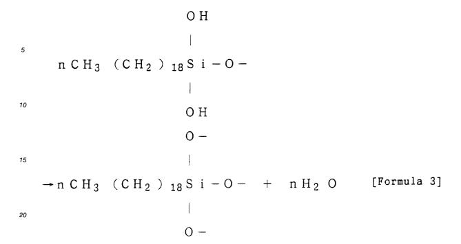
With this series of operations, an organic coating film comprising nonadecyl-trichlorosilane was formed on the silicon substrate. It had a thickness corresponding to the molecular length of the surface active material (i.e., 2.5 nm).
