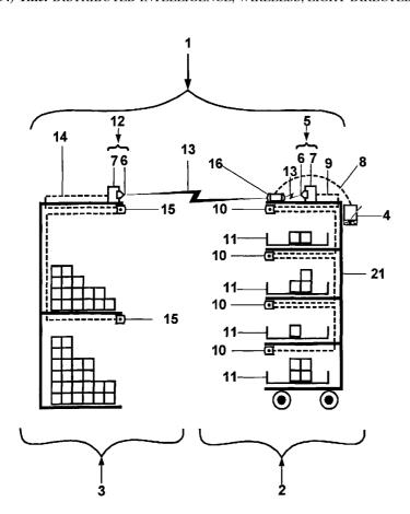
(57) Abstract: A system by which a portable computer (4) on a cart (2) translates warehouse locations to light addresses of locations on storage bays (3) in a storage facility and communicates instructions by means of a bi-directional, dual transmitter/receiver element (16) on the cart to a pick-controller unit positioned on each bay.
