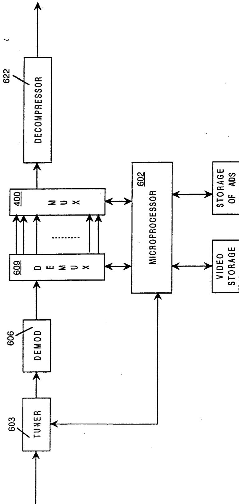
S TT CHANNEL SWITCHING HARDWARE: CHANNEL SWITCHING
