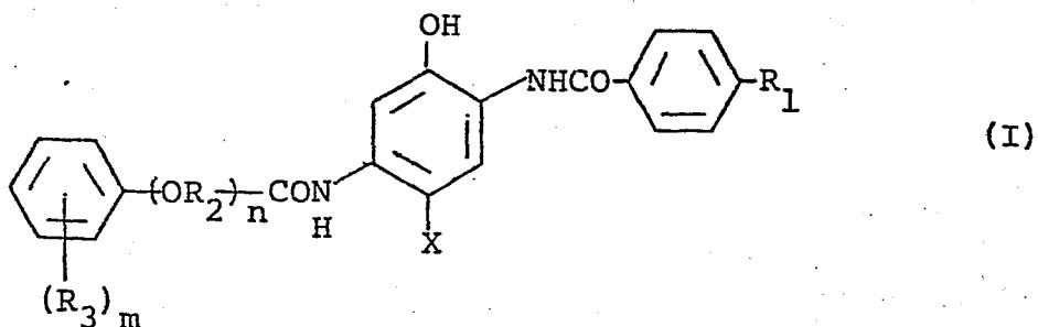
wherein  $R_1$  represents a branched chain alkyl group having from 3 to 4 carbon atoms;  $R_2$  represents an alkylene group having from 1 to 21 carbon atoms;  $R_3$  represents a hydrogen atom, a halogen atom, a substituted or unsubstituted alkyl group, a substituted or unsubstituted aryl group,
