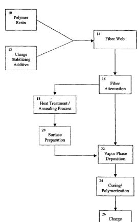
(57) Abstract: A vapor phase treated electret filter media includes an additive or mixtures thereof that enhance the charge stability of the media. The filter media achives acceptable alpha values for a range of filtration challenges without significant decay in alpha values over time. Preferred charge additives include fatty acid amides and mixtures thereof. Exemplary vapor phase deposition monomers include fluorinated monomers.
