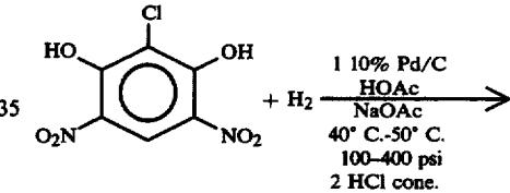
35  $\text{HO}-\text{C}_6\text{H}_3(\text{NO}_2)_2-\text{Cl} + \text{H}_2 \xrightarrow[\text{2 HCl cone.}]{\substack{10\% \text{Pd/C} \\ \text{HOAc} \\ \text{NaOAc} \\ 40^\circ \text{C.}-50^\circ \text{C.} \\ 100-400 \text{ psi}}}$
