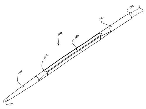
(57) Abstract: A linear sugical needle (100) is provided having a body portion including a proximal end section (110); a central section (13); and a distal end section (120). This distal end section has a substantially parabolic configuration for producing a substantially uniform stress profile along a length thereof.
