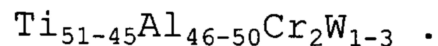
4. A Chromium and tungsten modified titanium aluminum alloy consisting essentially of titanium, aluminum, chromium, and tungsten in the approximate 20 atomic ratio of:
