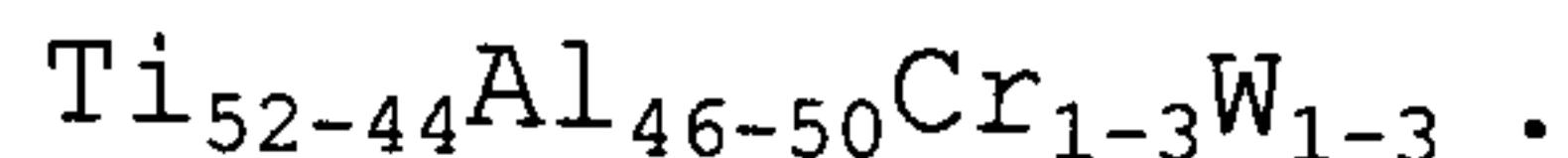
2. A chromium and tungsten modified titanium aluminum alloy consisting essentially of titanium, aluminum, chromium, and tungsten in the approximate 10 atomic ratio of:
