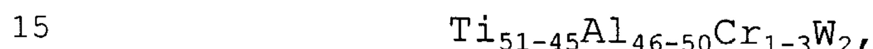
said alloy having been prepared by ingot metallurgy, and said alloy being given a heat treatment between 1250° C. and 1350° C.
