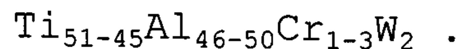
3. A chromium and tungsten modified titanium aluminum alloy consisting essentially of titanium, aluminum, chromium, and tungsten in the following 15 approximate atomic ratio:
