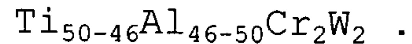
5. The alloy of claim 1, said alloy having been prepared by ingot metallurgy.
