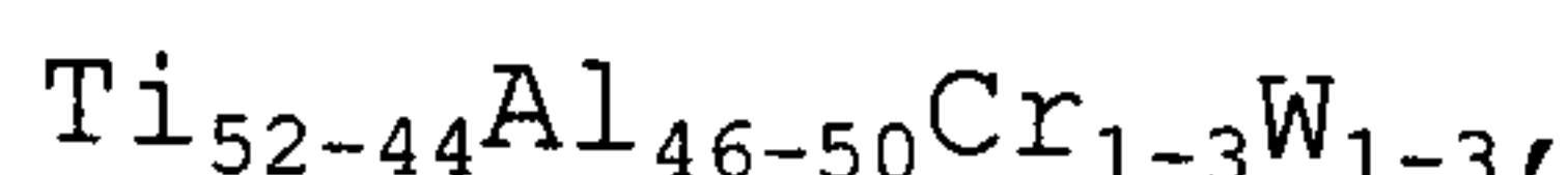
said alloy having been prepared by ingot metallurgy, and said alloy being given a heat treatment between 1250° C. and 1350° C.
