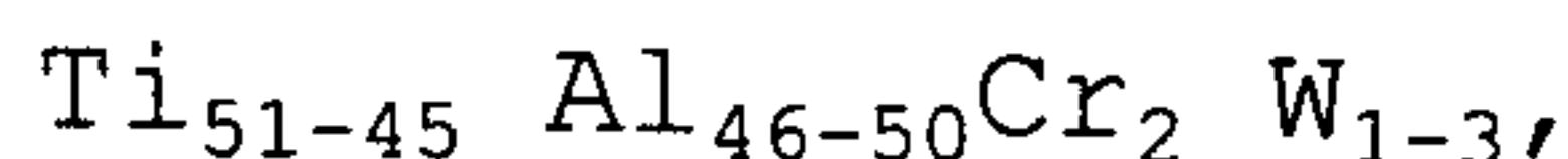
20 said alloy having been prepared by ingot metallurgy, and said alloy being given a heat treatment between 1250° C. and 1350° C.
