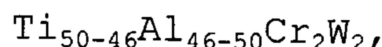
5 said alloy having been prepared by ingot metallurgy, and said alloy being given a heat treatment between 1250° C. and 1350° C.
