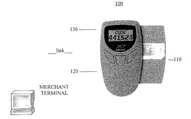
All-In-One Xiring device (with on/off feature and CAP feature) having PayPass functionality. The device has a PIN CVR "indicator" to merchant POS components. The device provides a new PIN management feature and re-uses current message infrastructure where the merchant terminal receives a transaction that has already been approved (signed) by the consumer.
